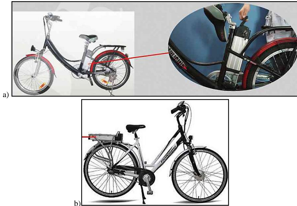
Fig. 4 Possible mounting places for the battery [13]
